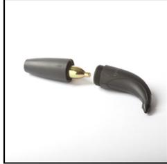
Unscrew cup of filler, and place CO<sub>2</sub> cartridge inside. Screw cup onto body of filler finger tight, then twist approximately another half-turn to puncture seal of cartridge. The gap between cup and body is normal.
